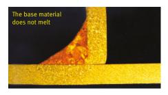
Using copper-based additives (bronze) means that less heat can be applied. Because less heat is applied, very little zinc vaporises and component distortion is reduced.
