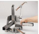
▶ The third clamping arm can be simply rotated out
