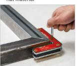
Hexagon hole for releasing the magnetic bracket
