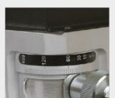
Continuously adjustable angle adjustment from 15°-180°
