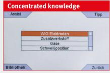
▶ A library ensures that setting up is child's play. This guarantees a fast and easy selection for both simple and complex welding tasks. Setup via selection of the basic material, the weld form and material thickness.
