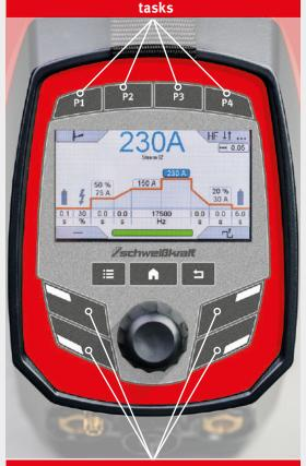
Fast and easy storing of four current welding
