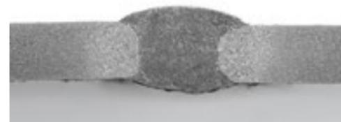
Optimum, slightly rounded weld appearance without fusion defects – for maximum gap tolerance and gap bridging.
