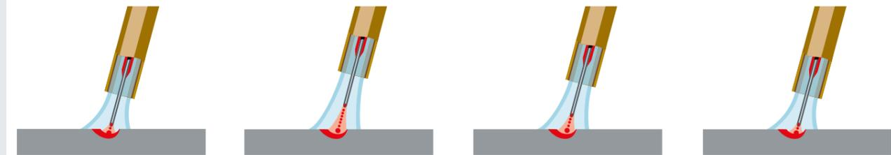
The new S series affords the welder intuitive ease of use that is combined with a clearly improved control over the pulse arc and allows him to react much more easily to arising conditions by adjusting the distance of the torch while welding. Whether you are dealing with varying gap dimensions or unevenness in the workpiece – even cumbersome welding positions, e.g. in corners, will be much easier to master.
