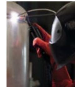
The **automatic cold wire feeder Lorch Feed** automates the manual feeding of filler material.
