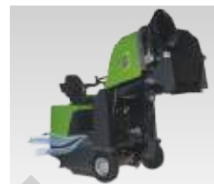
Hydraulic emptying of waste container up to a height of 1.4 m.
