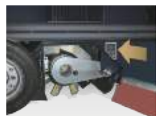
Main sweeping roller can be replaced without tools. Pressure and height setting of main sweeping roller separately adjustable
