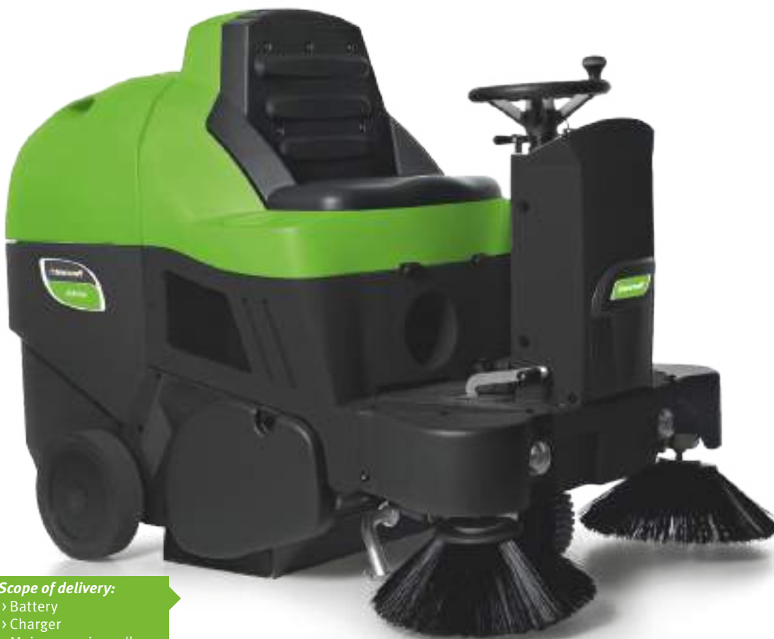
Central and side brushes can be replaced without tools
