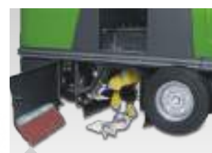
Main sweeping roller and side brushes can be replaced without tools
